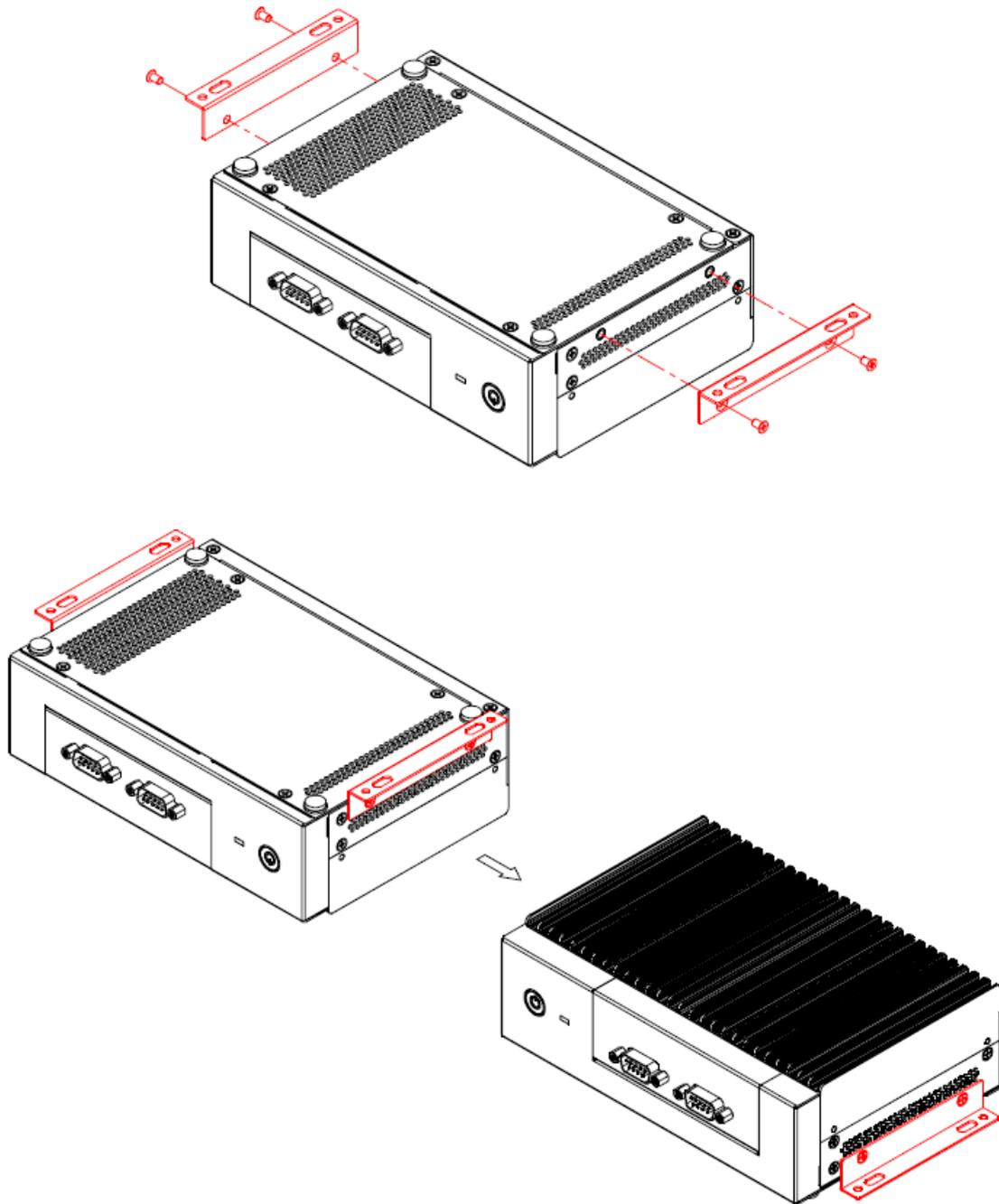
**Step1.** Fasten four M3\*5 screws on each side of the system to secure Mounting brackets.
