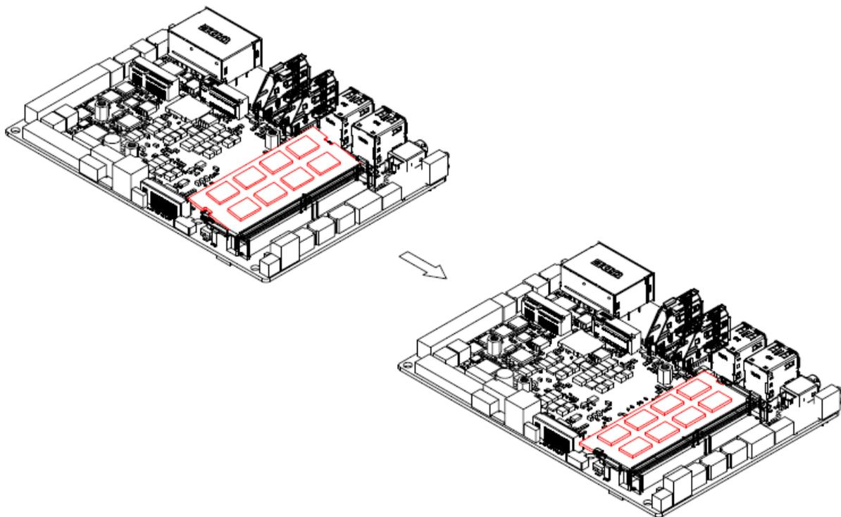
**Step5.** Slide the DDR4 SODIMM into the memory socket and press it down until properly seated.
