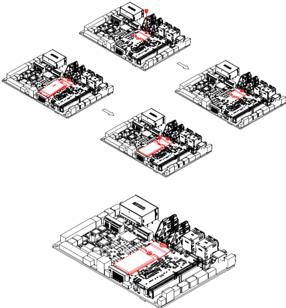
**Step1.** Fix bracket (24.6\*22\*3) and standoff screw with M3\*4 screw.
