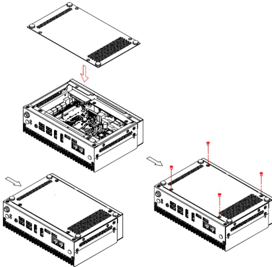
**Step4.** Put the bottom back and fix with four M3\*5 screws.
