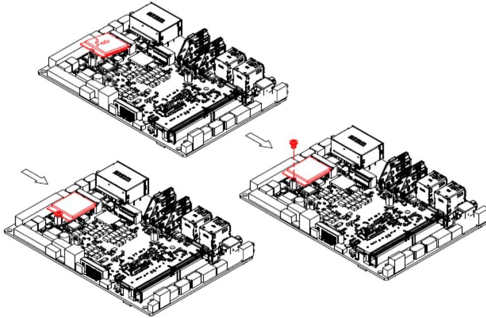
**Step1.** Insert M.2 E-Key card into designated locations and fasten with M3\*4 screw to complete installation.
