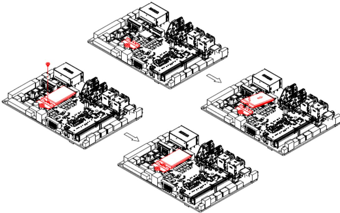
**Step1.** Fix bracket (16.6\*22) and standoff screw with M3\*4 screw.
