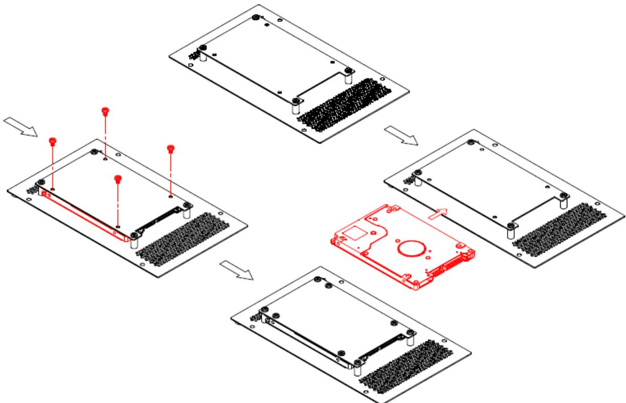
**Step2.** Install HDD.
