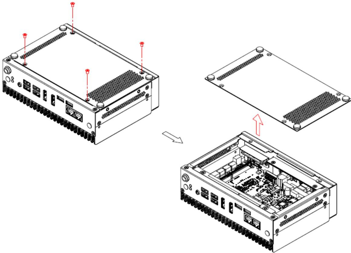
**Step1.** For HDD installation, remove four M3\*5L screws from bottom cover.
