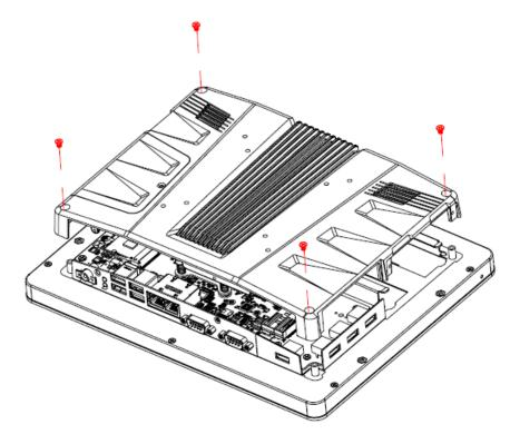
Step 2. Remove 4 screws to release the chassis cover, and remove it.
