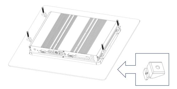
**Step 4.** Insert the hook brackets into the mounting bracket's hole, and then tighten the screws to affix the panel PC in place, fasten all the hook bracket to ensure panel PC well fix at cabinet.
