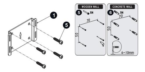
**Step 2.** Select the location on the wall for the wall mount plate, secure the mount plate to the wall by inserting four M5 screws into pilot holes and tightening them.
