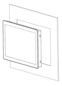
**Step 1.** Prepare a panel cutout according to the panel PC dimensions. For the panel cutout dimension, please refer to "System Dimensions" section in this manual.
