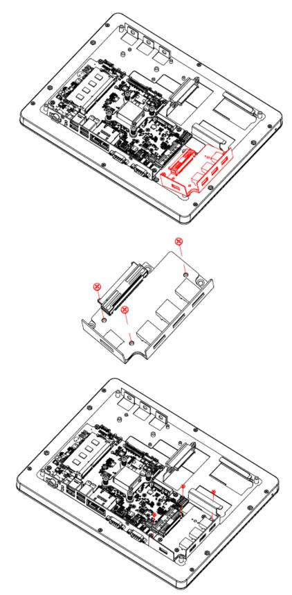
**Step 3.1** Insert the ARC-BYT DB into the socket and fasten 3 screws. **Step 3.2** Re-assemble your system back through previous steps to complete the installation.
