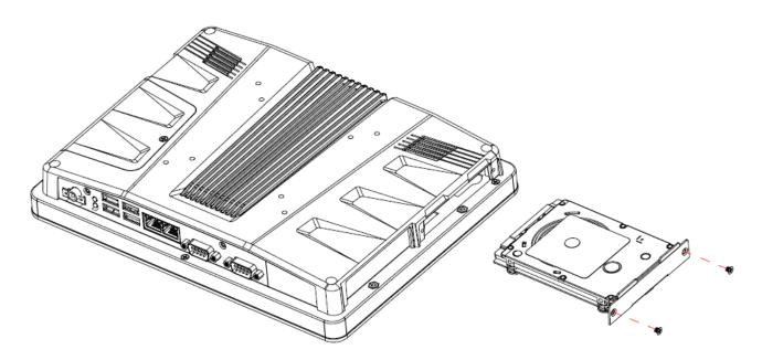
Step 3. HDD Installation: Insert the HDD into the Drive Bay and fasten 2 screws.
