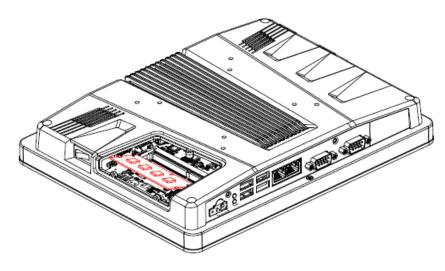
**Step 2.1** Insert the SODIMM into the memory socket.
