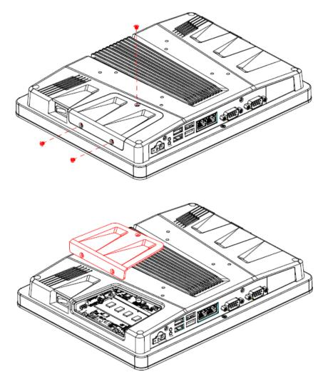
Step 1. Memory Installation: Remove 3 screws to release the chassis cover, and remove it.
