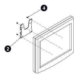
**Step 1.** Insert four M4 screws into the VESA holes on the panel PC and tighten them to secure the bracket to the rear panel, ensure that the thread depth of the screws on the rear panel does not exceed 4mm.
