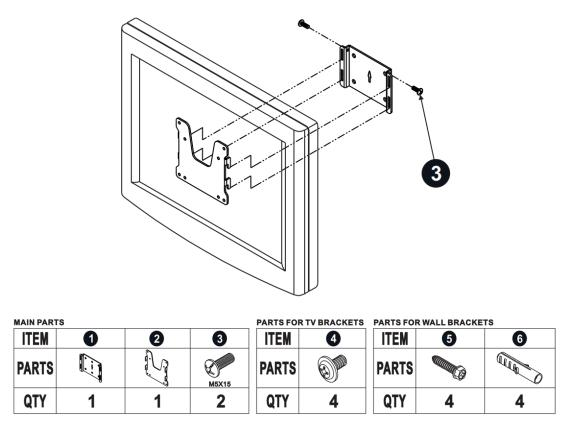
**Step 3.** To mount the panel PC on the wall, align the wall mount bracket attached to the panel PC with the wall mount plate on the wall and slide the panel PC downwards to hang the bracket on the mount plate. Secure the panel PC in place by tightening screws in the wall mount bracket.
