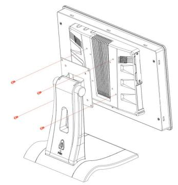
**Step 1.** Refer to the installation instruction of mounting arm/ stand to correctly assembly the arm/ stand onto the surface as a base.
