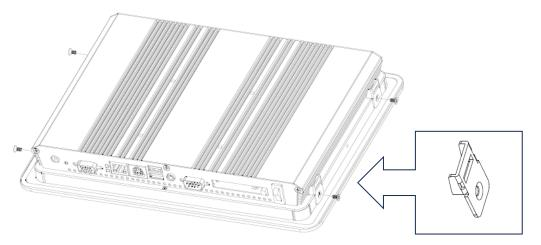
Step 2. Add mounting brackets and fasten screws into the frame.
