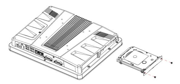
Step 1. Unfasten 2 screws of the HDD bracket and take it off.
