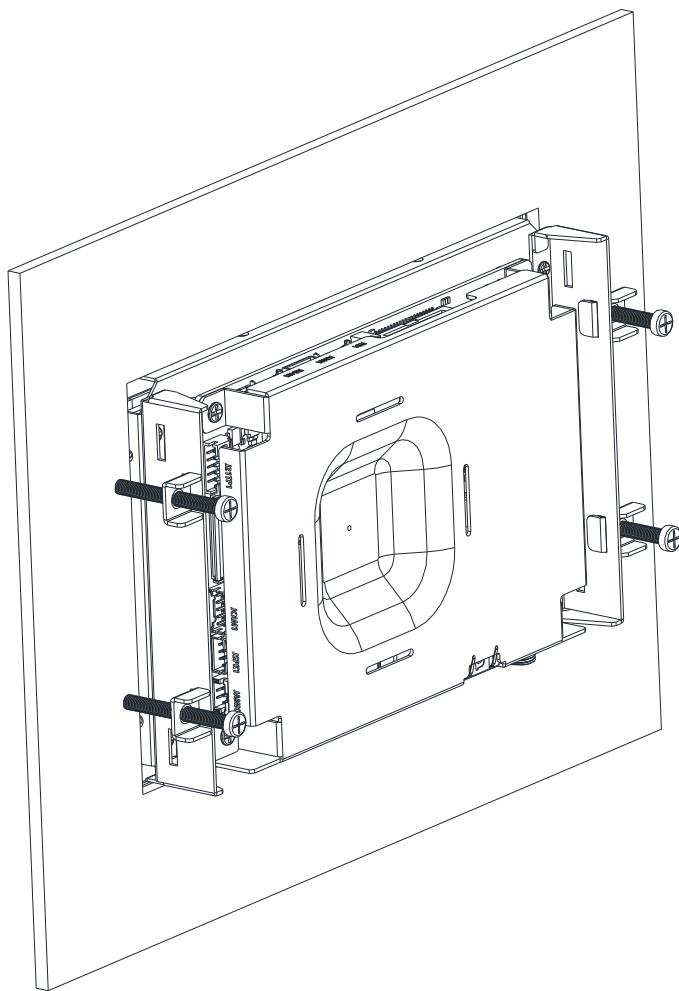
**Step4.** Insert and fasten 4 Panel mount screws to secure the module.
