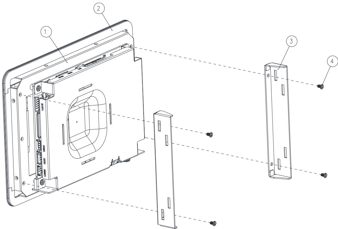
**Step1.** Insert and fasten 4 screws to secure Panel mount bracket.
