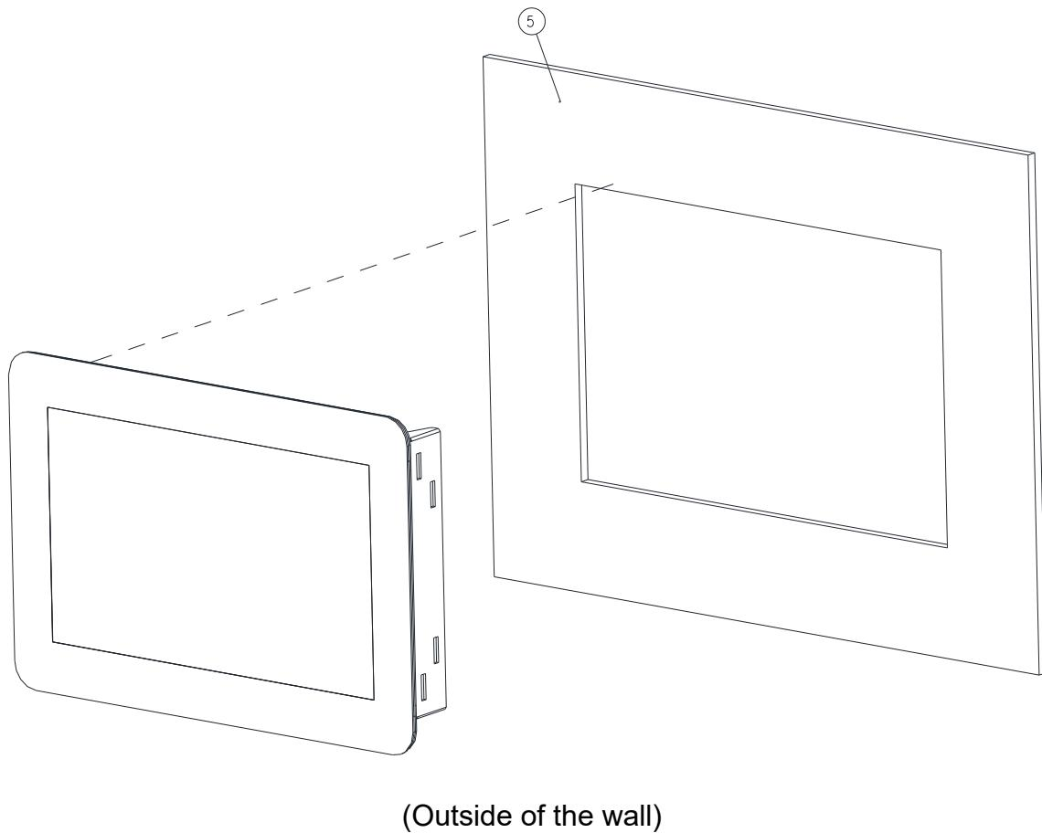
**Step2.** Insert OFT-07WR2 Open frame into the wall.
