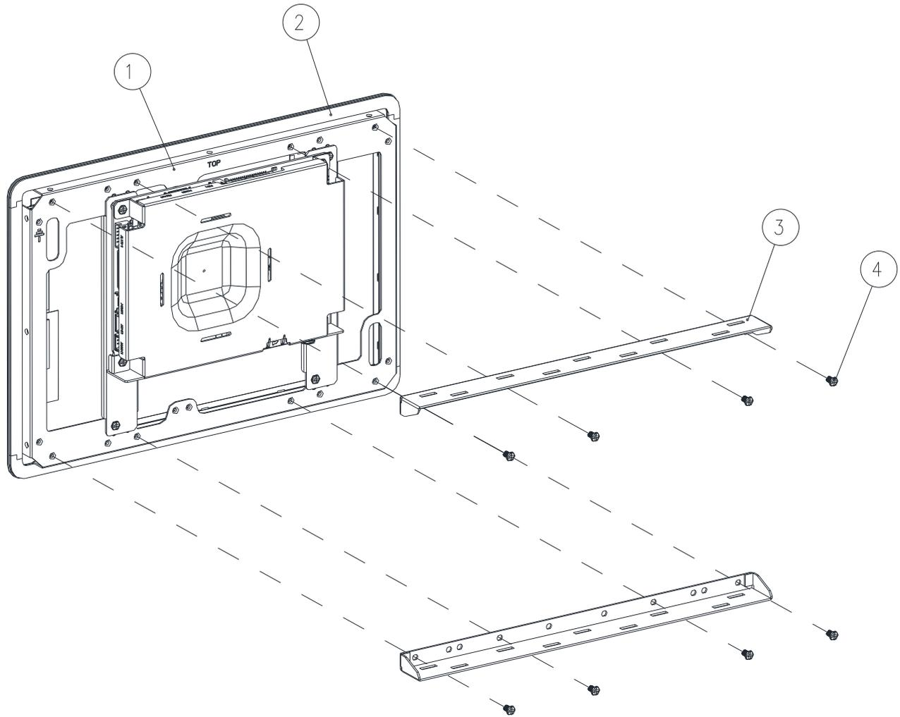
**Step1.** Insert and fasten 8 screws to secure Panel mount bracket.
