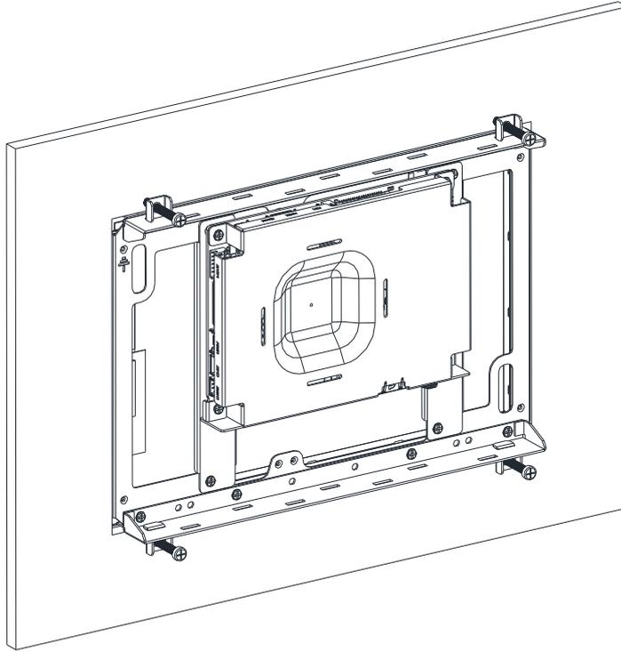
**Step4.** Insert and fasten 4 Panel mount screws to secure the module.
