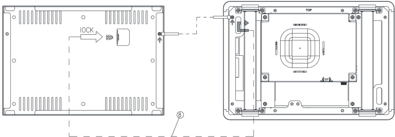
**Step4.** Wrap the Kensington lock (option) around the hole in the OFT-10WR2 and attach the lock to the keyhole in the Wall box.
