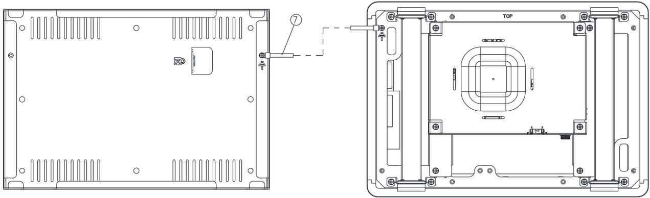
**Step3.** Fasten the Ground wire with 2 screws on the ground screw holes of OFT-10WR2 and Wall box.
