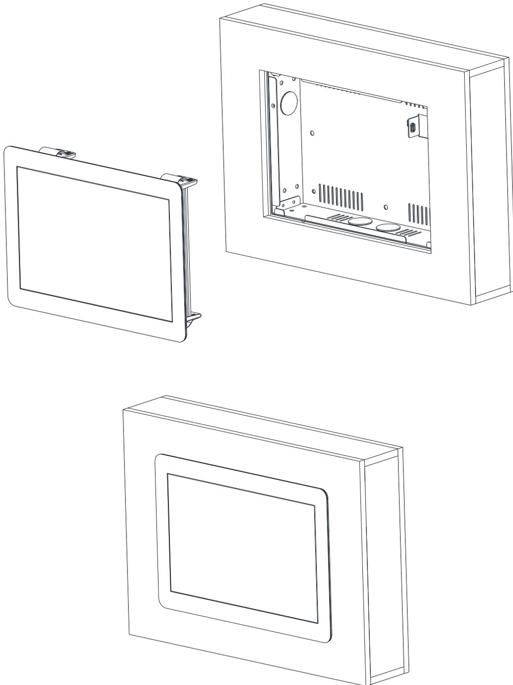
**Step5.** Store the Ground wire and Kensington lock in the Wall box and embed the OFT-10WR2 into the wall (Wall Box).
