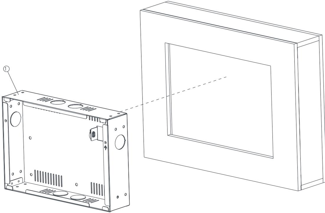
**Step1.** Install the 10" Wall Box and fix it on the wall, and use suitable screws to lock the wall box (the screws can be purchased according to actual needs)
