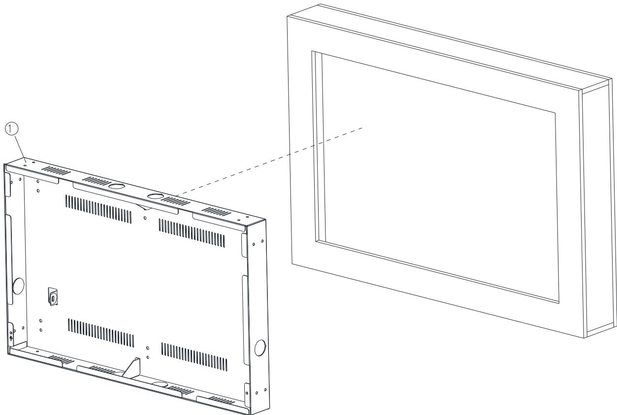
**Step1.** Install the 21" Wall Box and fix it on the wall, and use suitable screws to lock the wall box (the screws can be purchased according to actual needs)
