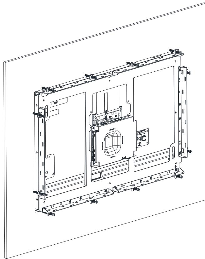
**Step4.** Insert and fasten 12Panel mount screws to secure the module.
