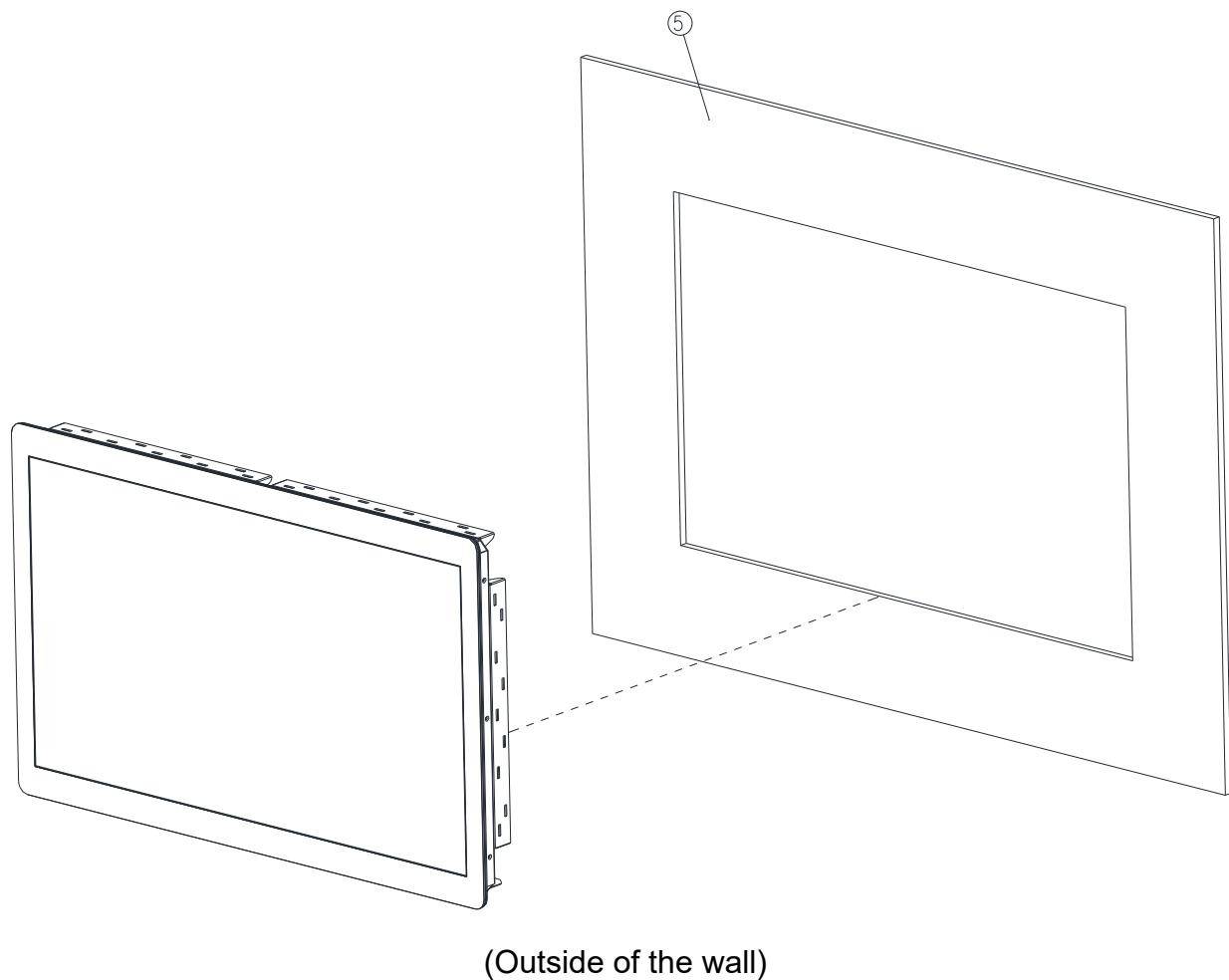
**Step2.** Insert OFT-21WR2 Open frame into the wall.
