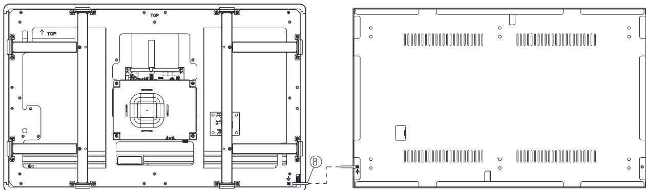
**Step3.** Fasten the Ground wire with 2 screws on the ground screw holes of OFT-21WR2 and Wall box.
