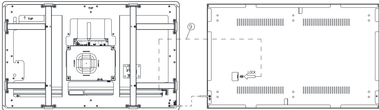
**Step4.** Wrap the Kensington lock (option) around the hole in the OFT-21WR2 and attach the lock to the keyhole in the Wall box.
