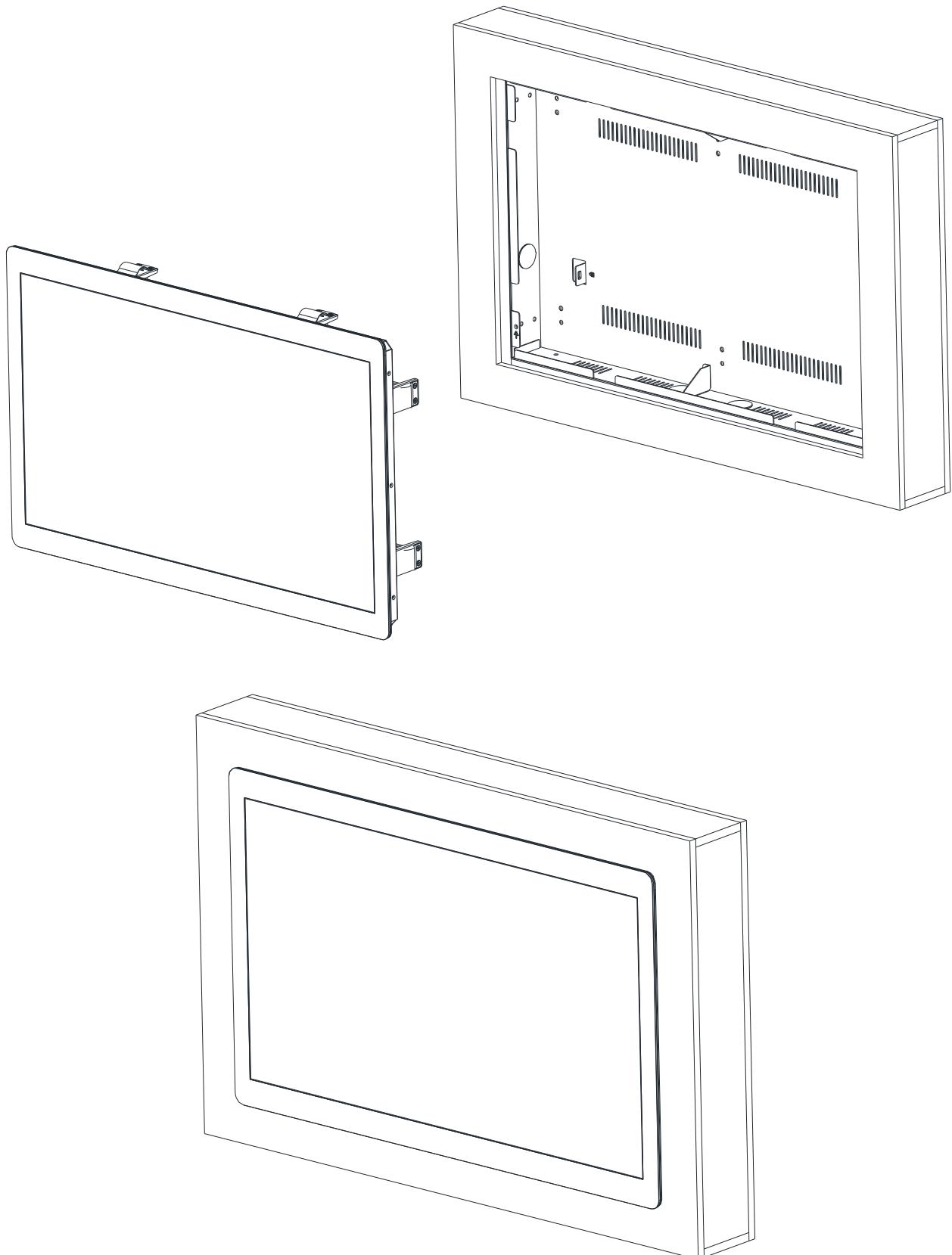
**Step5.** Store the Ground wire and Kensington lock in the Wall box and embed the OFT-21WR2 into the wall (Wall Box).
