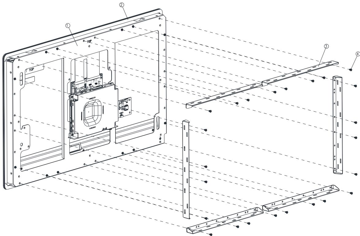
**Step1.** Insert and fasten 24 screws to secure Panel mount bracket.
