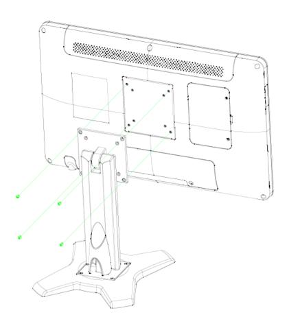
**Step1.** Position VESA Mount on both sides, matching the holes on the system. **Step2.** Insert and fasten 4 screws on each side of the monitor to secure Mounting brackets.
