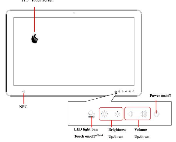
Note1: Press this button for 2 sec to turn on or off LED reading light bar Press this button for 4 sec to turn off or on for touch function
